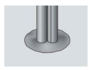
Fill up to the full thickness of the floor or wall (filling thickness 150 mm or more), and finish by smoothing the surface.
