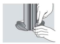
Get rid of dirt on the cables and opening, and fill up with the putty.
